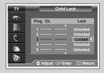
This feature allows you to lock the television so that it cannot be switched on via the front panel. It can, however, still be switched on via the remote control. Thus, by keeping the remote control away from unauthorized users, such as children, you can prevent them from watching unsuitable programme.
